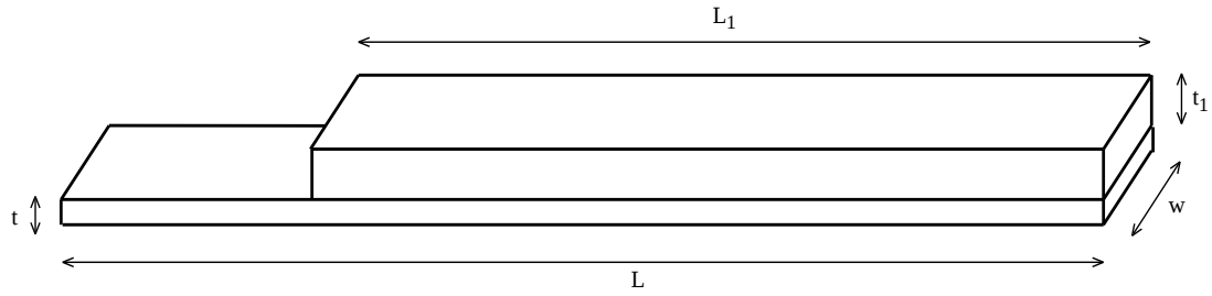
Figure 4.8 : Partially damped beam.
