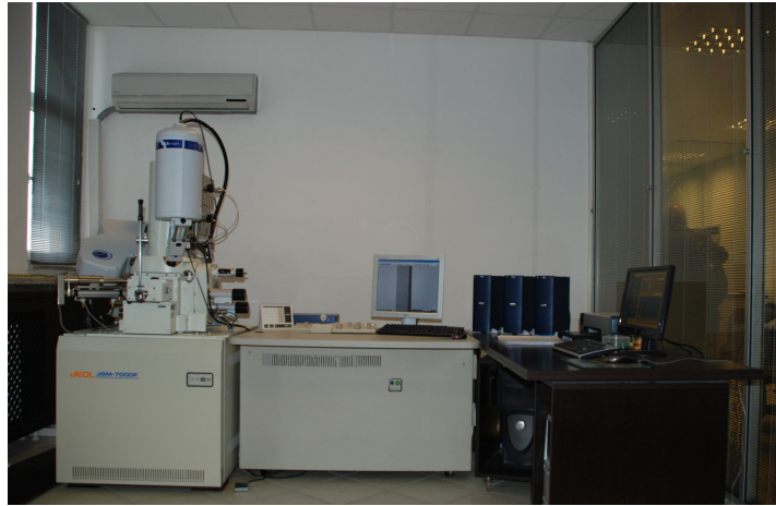
Şekil 4.9 : JEOL JSM 7000F Field Emission-Scanning Electron Microscope cihazı
