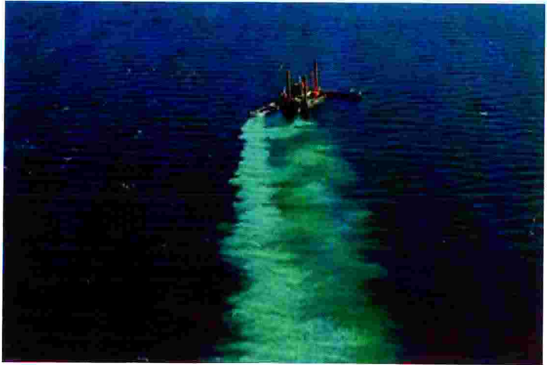
Figure 4.3 : Typical dredging operation in white limestone, Oeresund, Denmark. [1]
