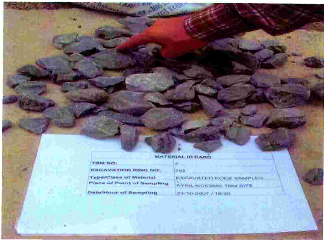
Figure 14-2 Samples from excavation of ring no 552
