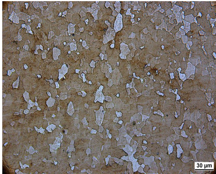
Figure A.5. Microstructure of Steel C, as-recieved (X500).
