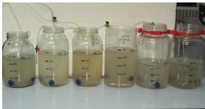
Figure 5.11: Reactors of inert COD analysis.
