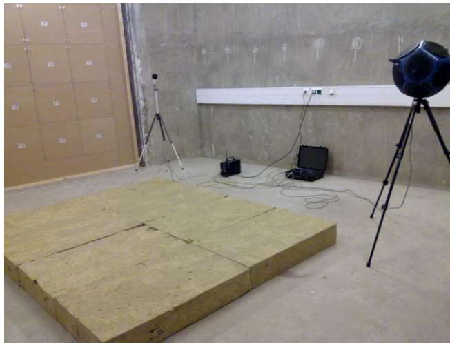
Figure 3.20: Rockwool plates and the measurement equipment in the laboratory.
