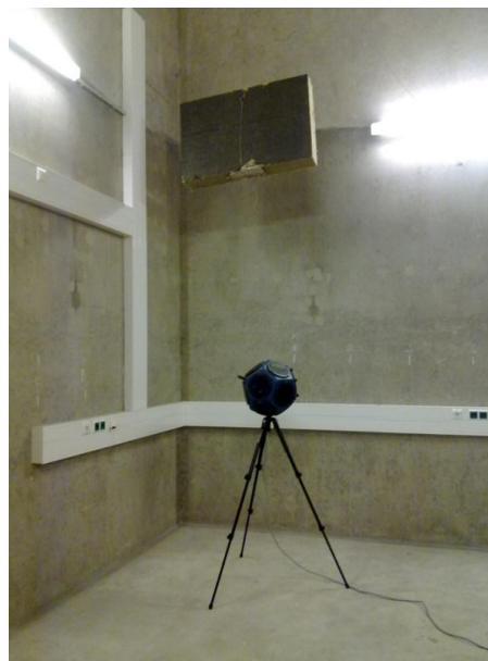
Figure 3.10: The omni-directional source and a rockwool panel.
