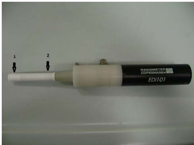
Figure 2.3: Working electrode 1)Removable tip 2)Rotating stem.
