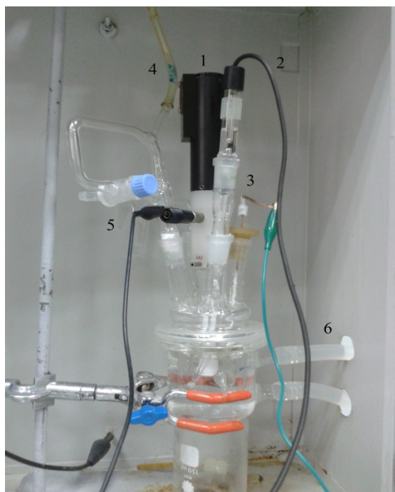
Figure 2.2: Glass cell with compartments: 1) Working electrode, 2) Reference Electrode, 3) Counter electrode, 4) Oxygen-Nitrogen inflow hose, 5) Oxygen-Nitrogen monitoring compartment, 6) Water jacket inflow-outflow hoses.
