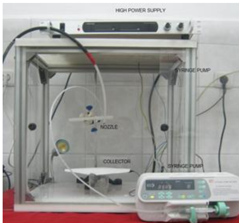
Figure 3.2 : Conventional electrospinning system.
