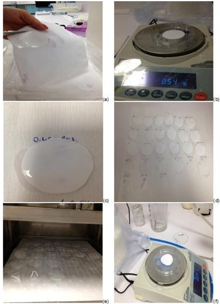
Figure 3. 9. Images of the porosity experiment.
