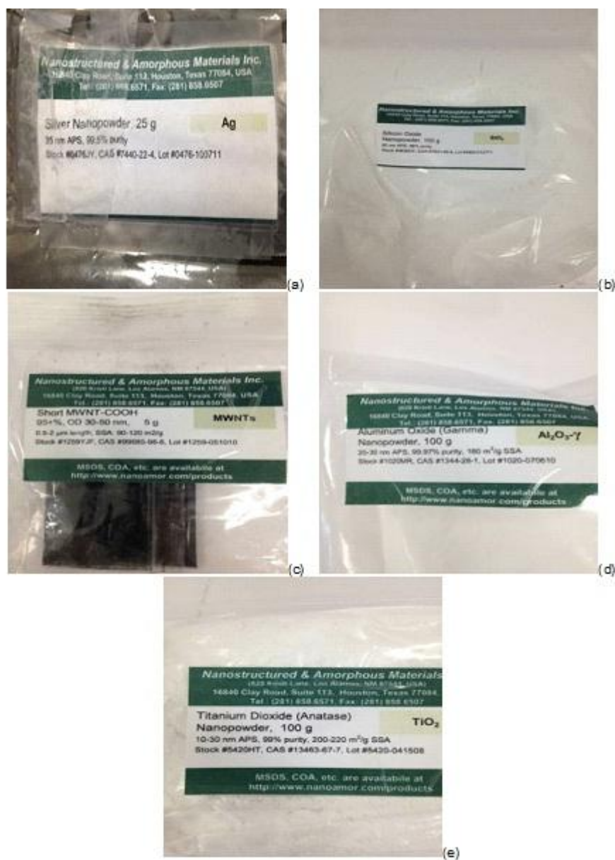
Figure 3. 2.Nanomaterials, used for producing the nanocomposite membranes (a) AgNP (b) SiNP (c) CNT (d) AlONP (e) TiNP.
