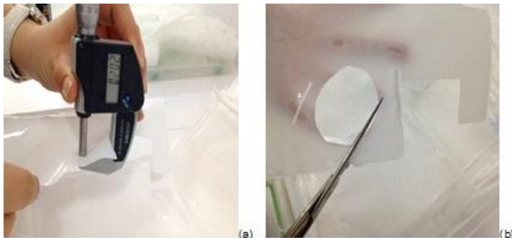
Figure 3. 6. Measurement of the membrane thickness.
