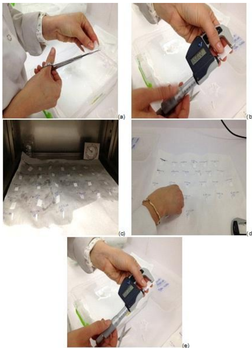
Figure 3. 10. Images of the shrinkage ratio experiment.
