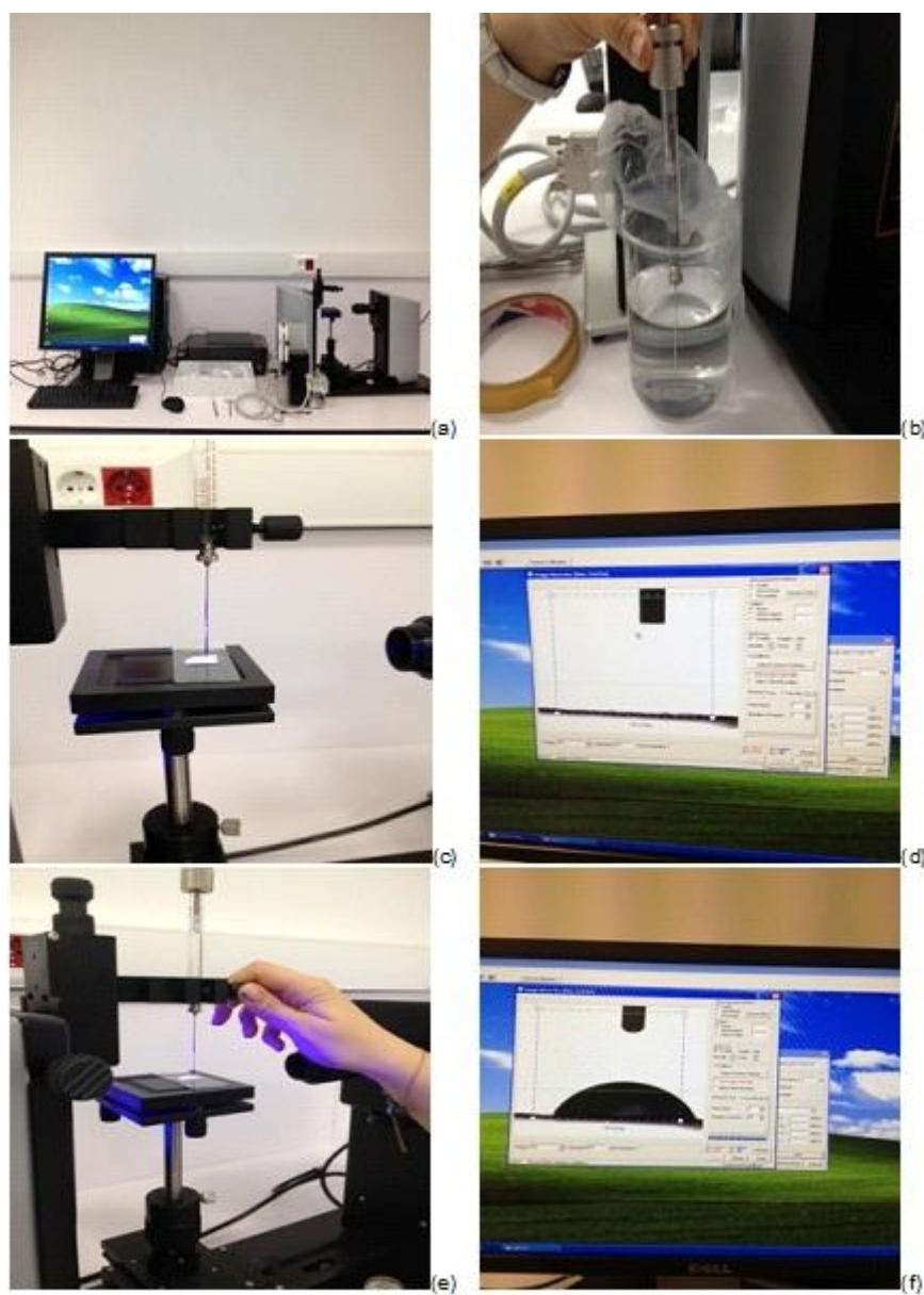
Figure 3. 11. Contact angle measurement device and the sample preparation process.
