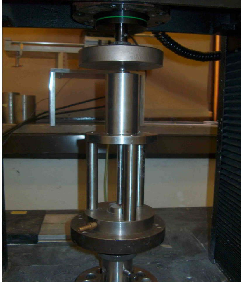
Figure A.1: Biaxial flexural strength test apparatus
