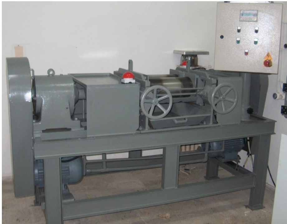
Figure 4.44: Calendering machine with two roller mills
