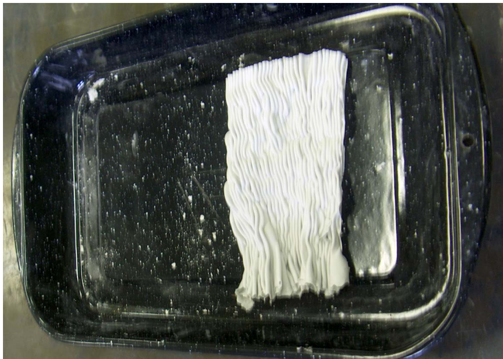
Figure N.4: MDF composite after high shear process
