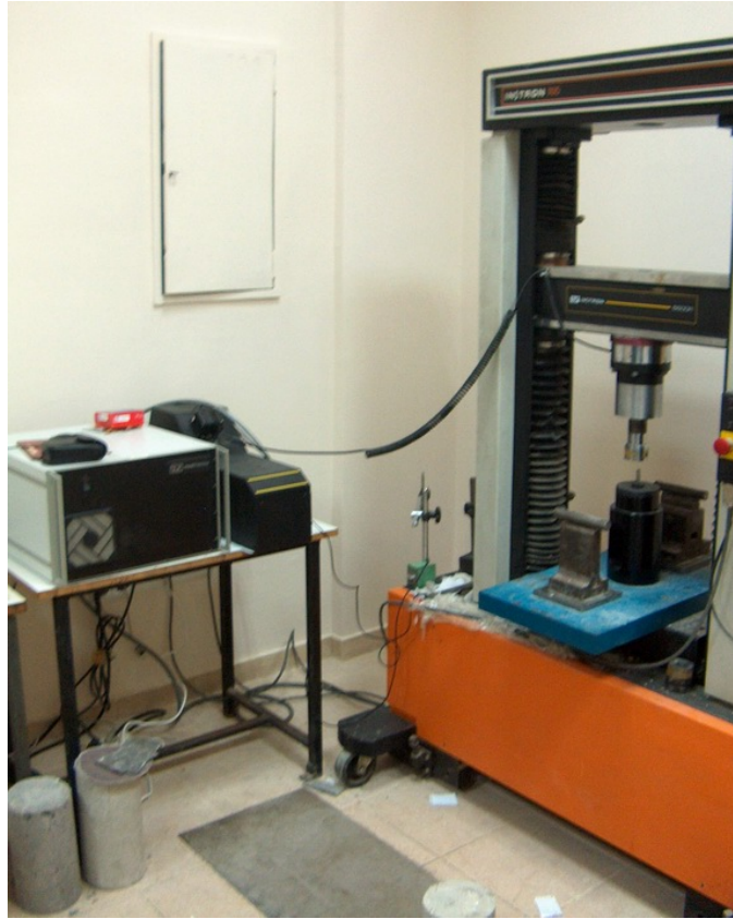
Figure 4.48: Biaxial flexural strength test setup
