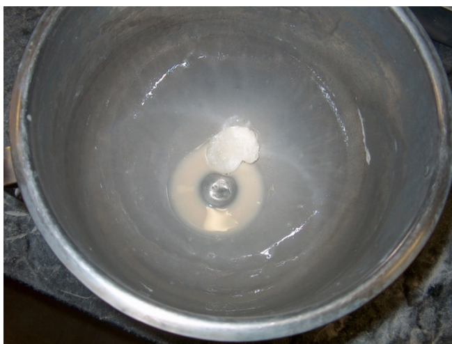
Figure 4.40: Mixing gel phase and \text{NaAlO}_2 +water mixture in a planetary mixer for mixture no. 9
