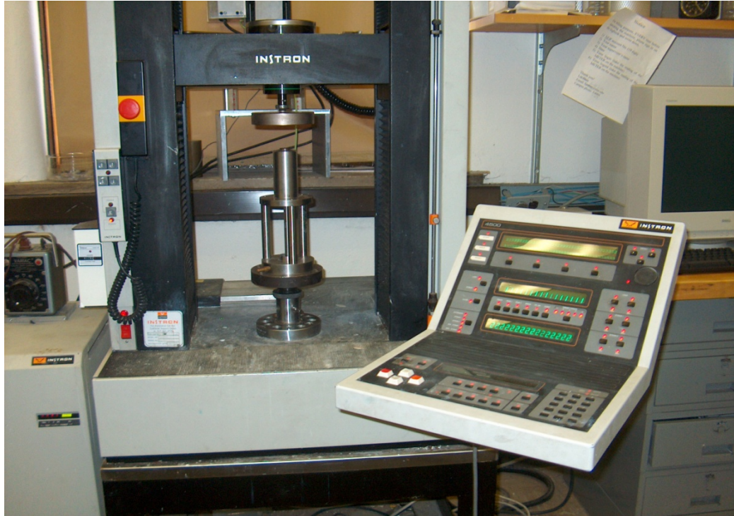
Figure N.7: Biaxial flexural strength test setup
