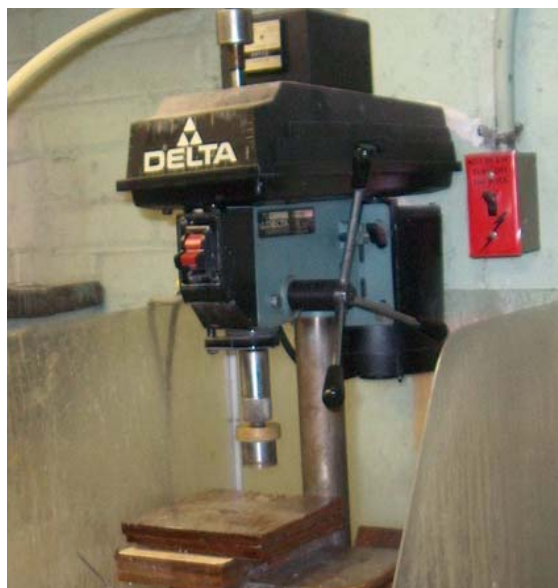
Figure 4.4: Core drilling machine used to prepare circular specimens from MDF sheets
