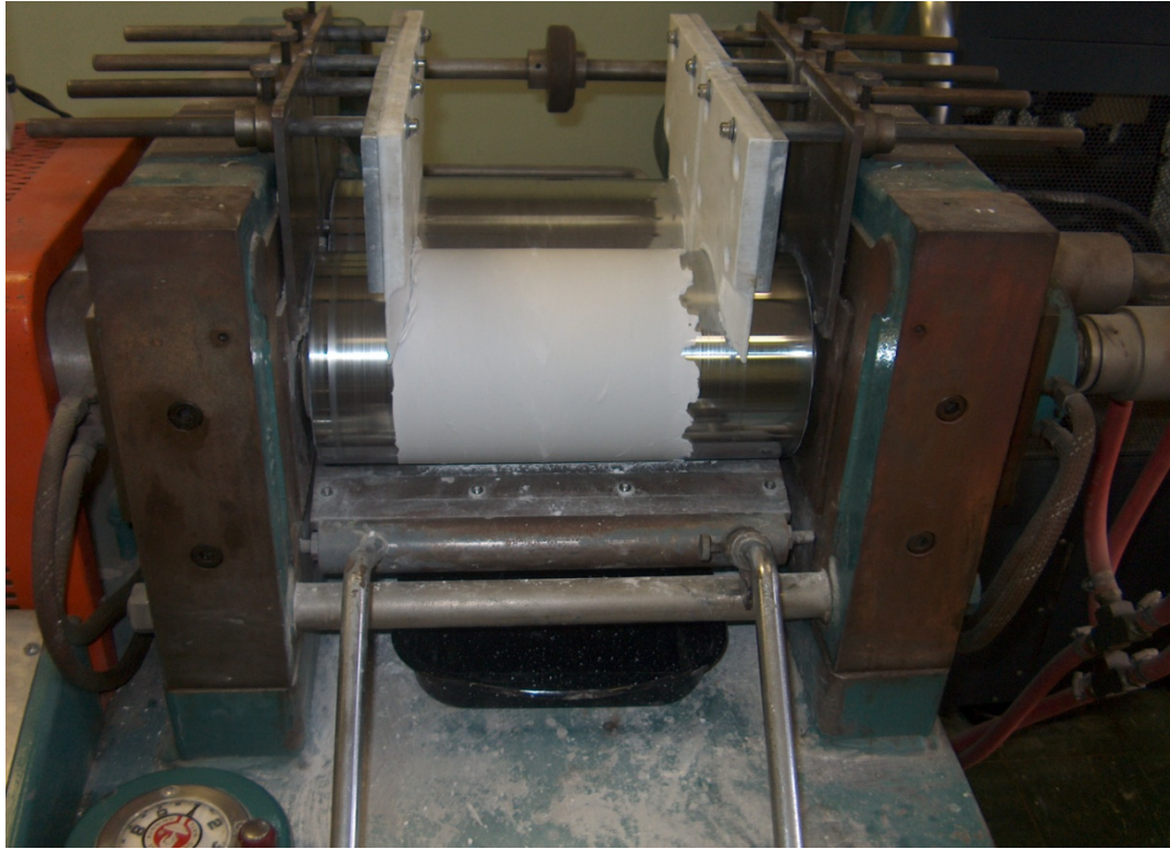
Figure N.3: MDF composite during high shear process
