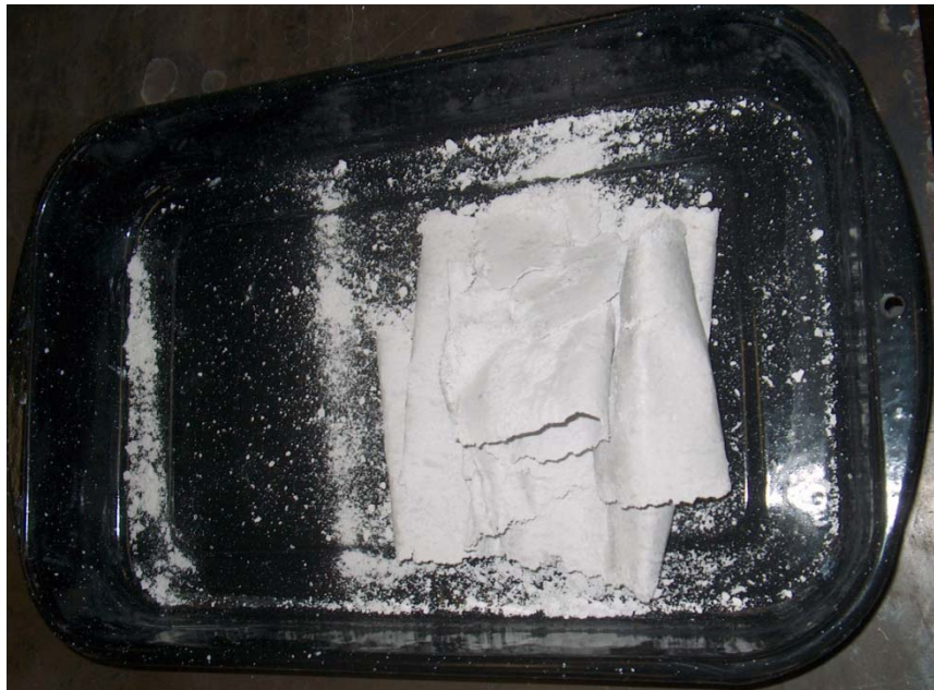
Figure N.2: MDF composite before high shear process
