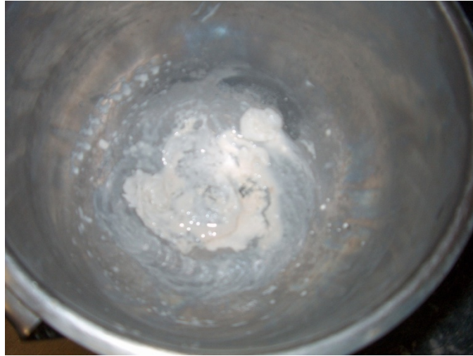
Figure 4.41: Mixing gel phase and \text{NaAlO}_2 in a planetary mixer for mixture no. 11
