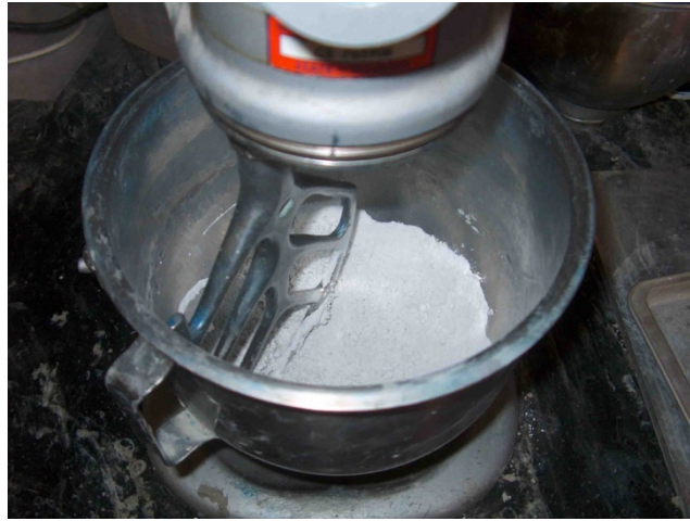
Figure 4.1: Mixing the materials in a planetary mixer
