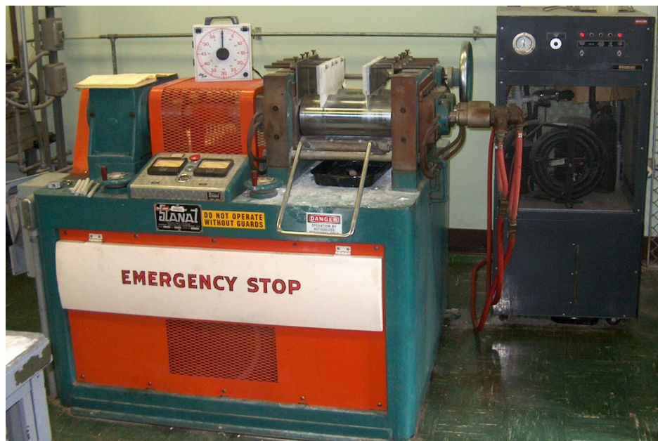
Figure 4.2: Calendering machine with two roller mills and cooling system
