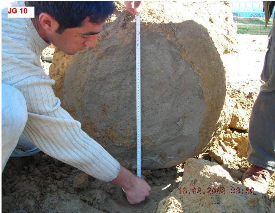
Figure 3.3: Test jet grout column.
