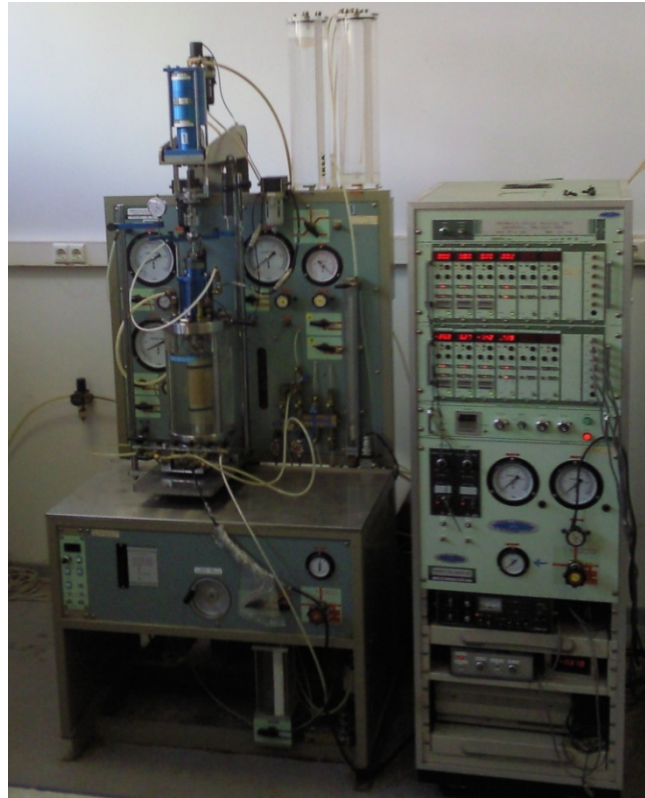
Figure 4.2 : Triaxial Test Apparatus in ITU Soil Dynamics Laboratory
