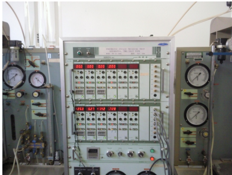
Figure 4.4 : Digital System of the Triaxial Apparatus
