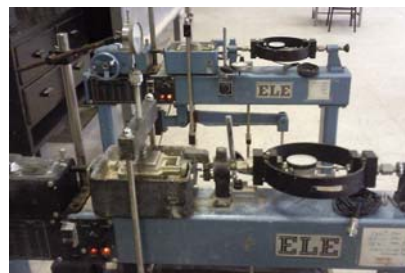
Figure 4.12 : Direct Shear Test Apparatus
