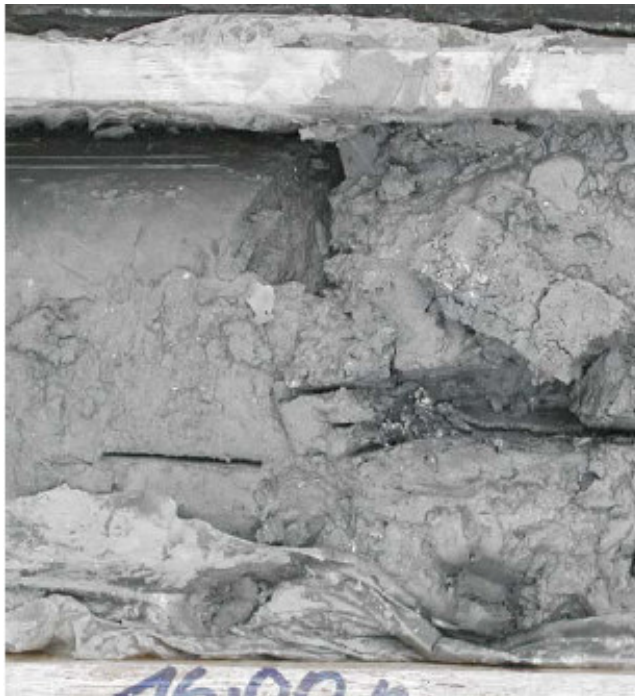
Figure 3.4 Drill core from the drilling in the Danube channel (clayey silt on the left, coarse silt on the right) (Martak and Herzfeld, 2005)
