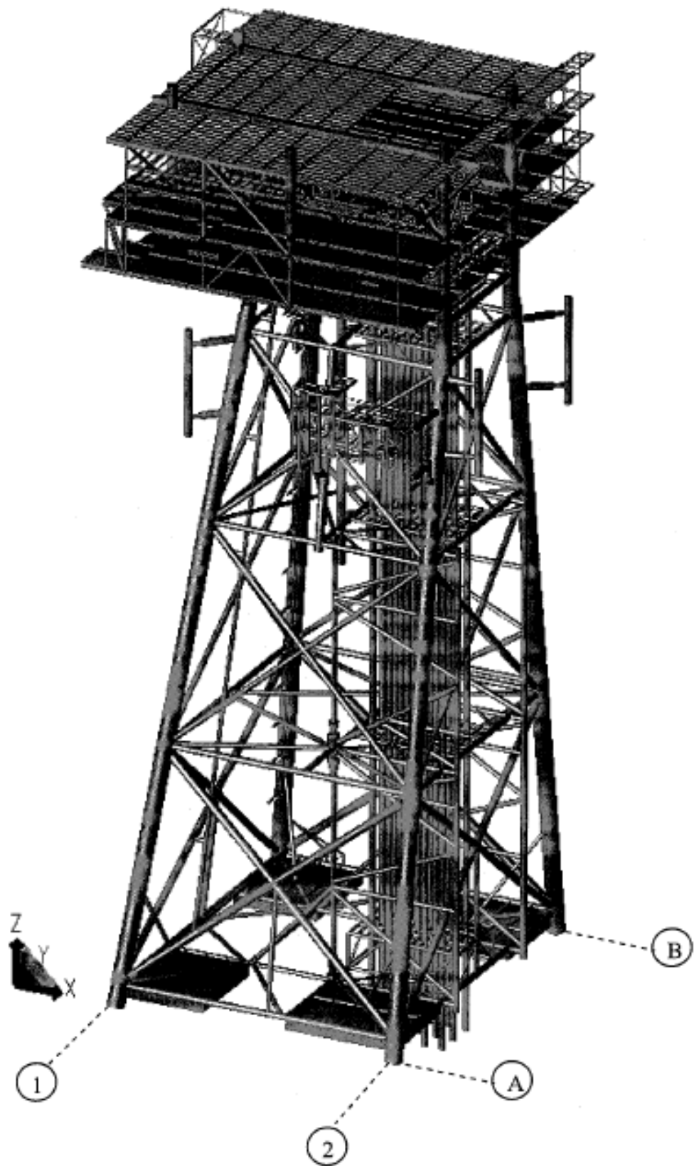
Figure 2.5 : SPD25 Wellhead Platform Topside, Jacket, and Substructures
