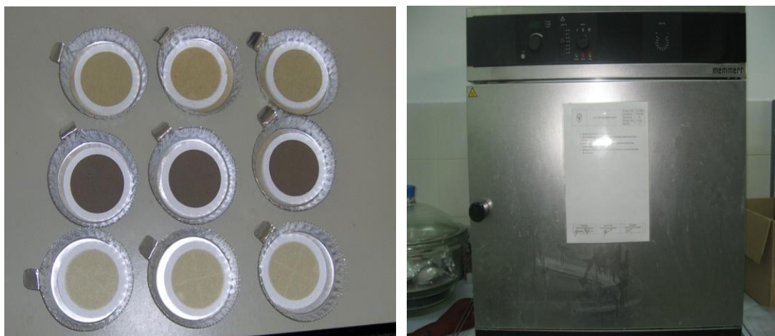
Figure 4.3: Left: Glass fiber filter disks sludge sample filtered; right: 105° C oven.
