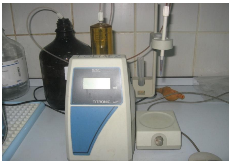
Figure 4.6: Titration for COD.
