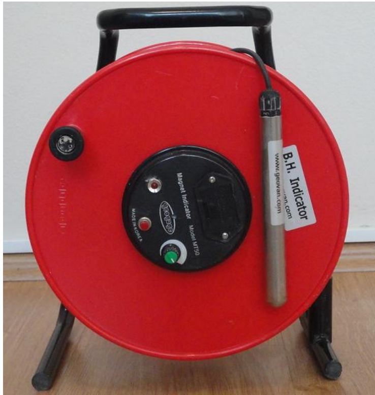
Figure 4.23: Magnet Reading Unit – Reed Switch Probe.
