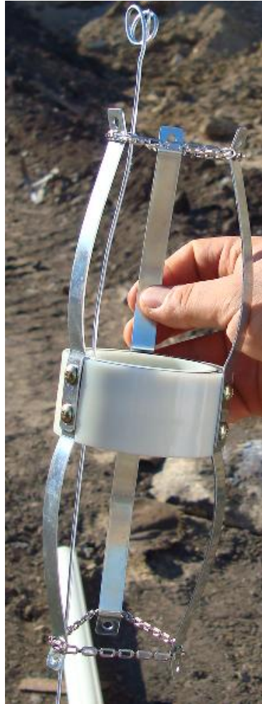
Figure 4.21: Spider Magnet attachment detail for Inclinator Casing.
