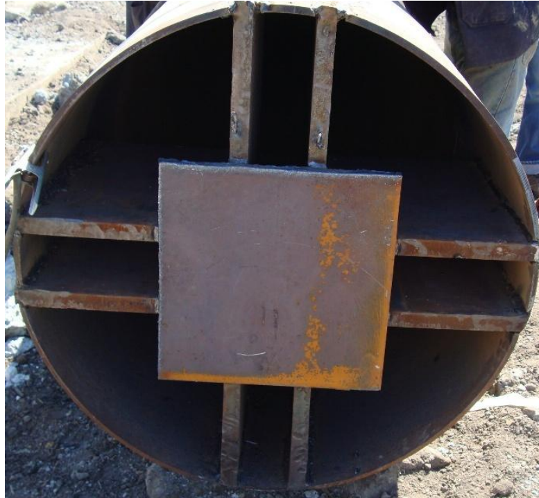
Figure 4.34: Plate between Load Cell and Steel Pipe.
