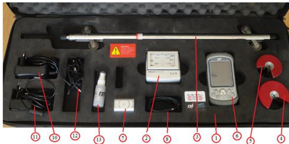
Figure 4.19: Parts of a Digital Inclinometer.
