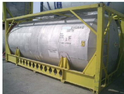
Figure 5.4: A tank container
