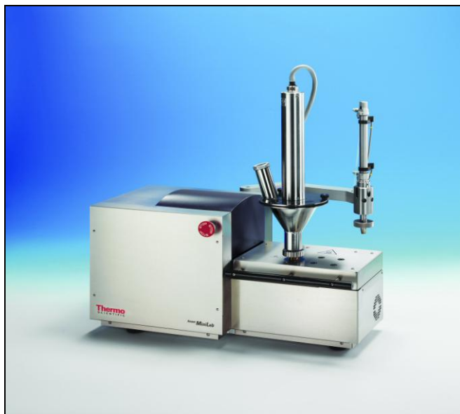
Figure 3.1: HAAKE MiniLab micro compounder.
