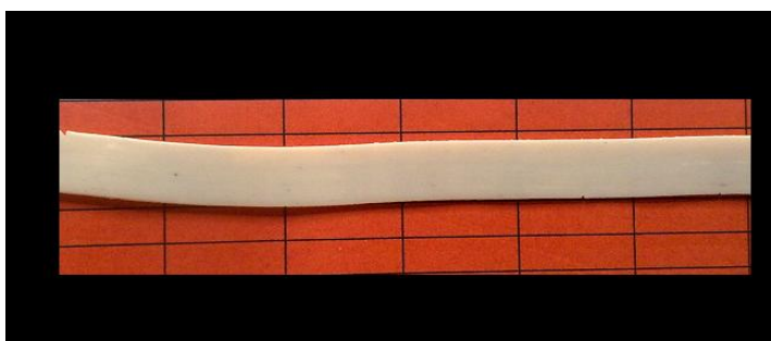
Figure 4.6 : Images of extruded tape sample (Piston diameter:12mm, app. 100 \text{ kg.cm}^{-2} ) of BP1/PS5 (40 w% BPS5)
