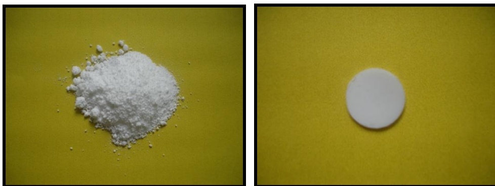
Figure 4.4 : Images of unprocessed and compression molded ( 100 \text{ kg.cm}^{-2} , 2 min) samples of BP3/ PS5 blend (40 w% PS5)
