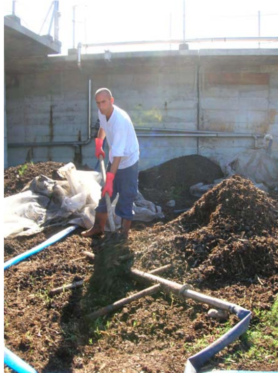
Photograph 3.10. Transferring the piles back on the ventilation system
