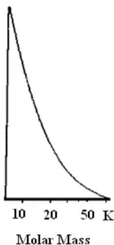
Figure 4.5: GPC trace of DADMAC-NVP (1:1) copolymer in water.
