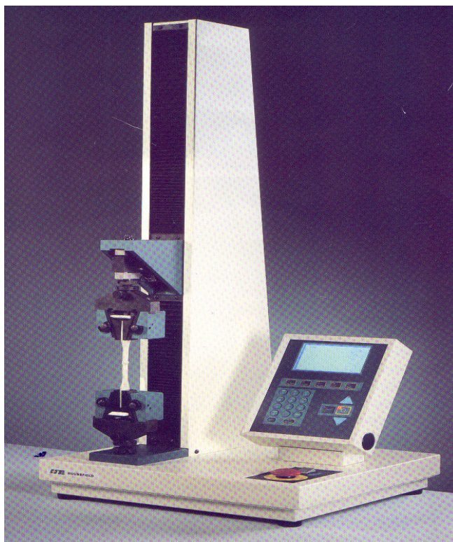
Figure 2.2: Hounsfield H5K-S model tensile testing machine
