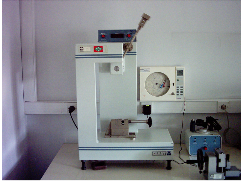
Figure 6.11. Ceast impact tester
