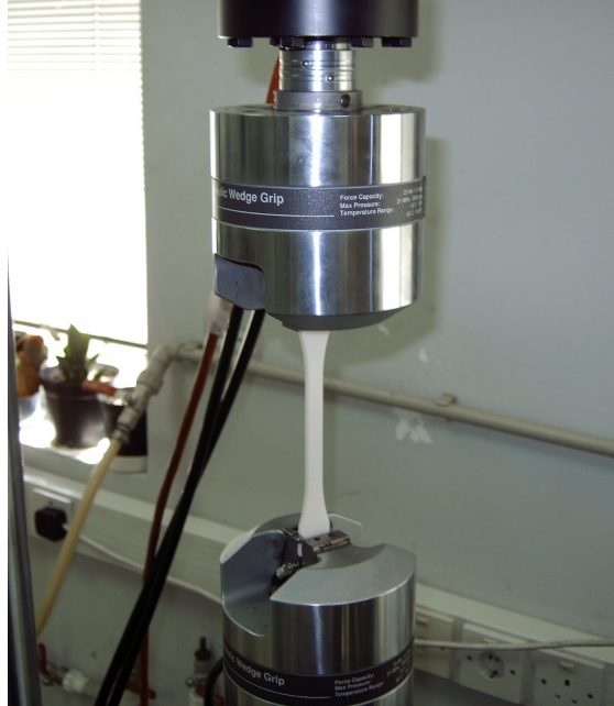
Figure 6.13. Hydraulic grippers of MTS fatigue testing system
