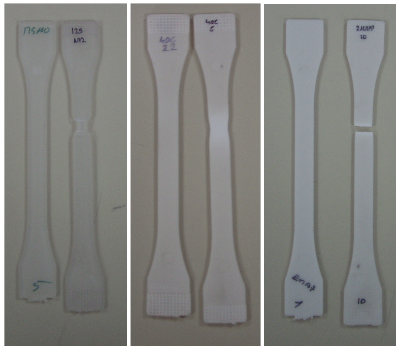
Figure 7.19. Fatigue test specimens after cyclic loading
