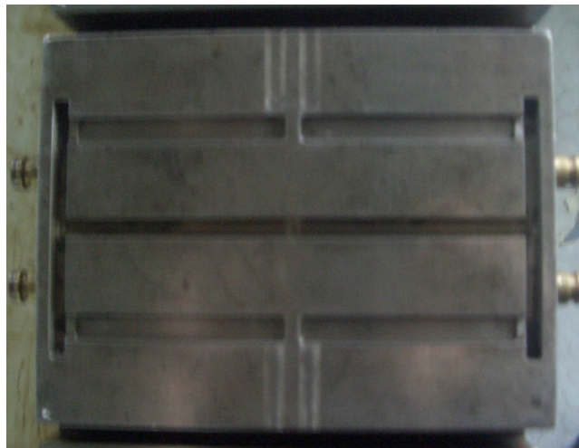
Figure 6.8. Impact test specimens mold ISO 178[36].
