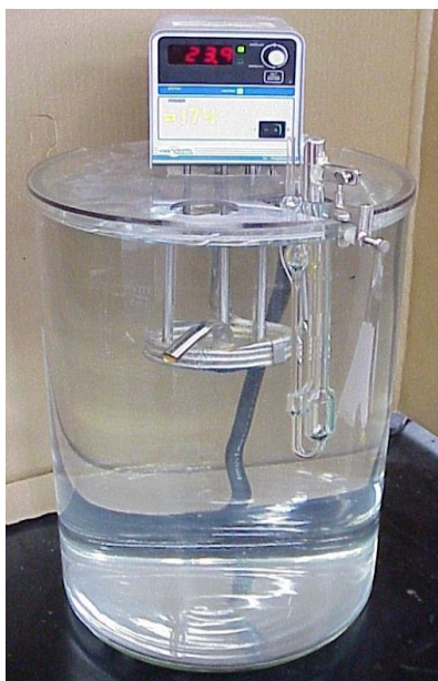
Figure 4. 1: The setup used for viscosity measurements consisting of Ubbelohde viscosimeter and temperature controlled water-bath.
