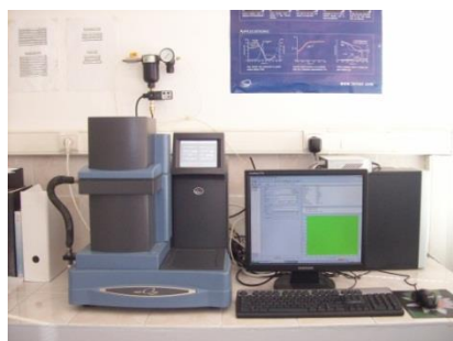
Figure 3.13: TA Q800 Dynamic Mechanical Analyser
