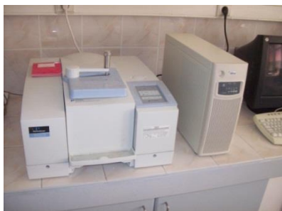
Figure 3.11: Perkin Elmer FTIR-ATR Spectrophotometer
