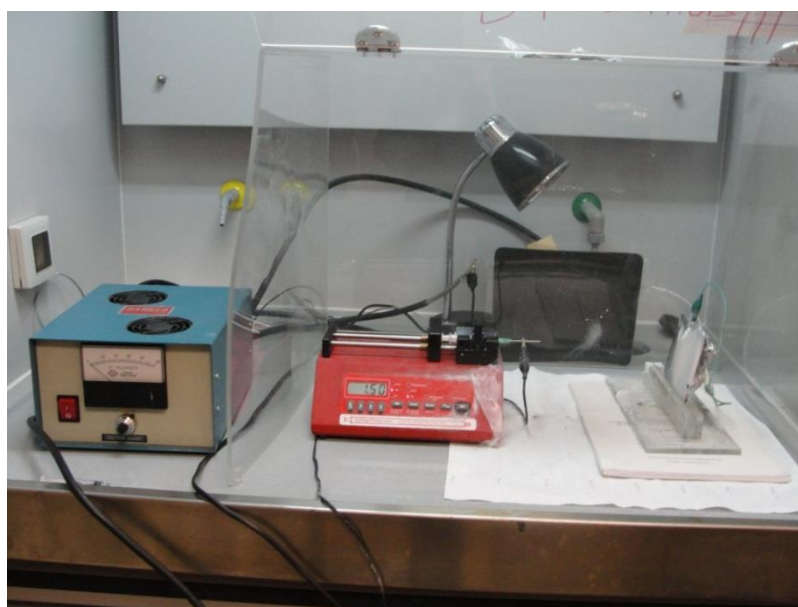
Figure 3.10: Experimental setup of electrospinning
