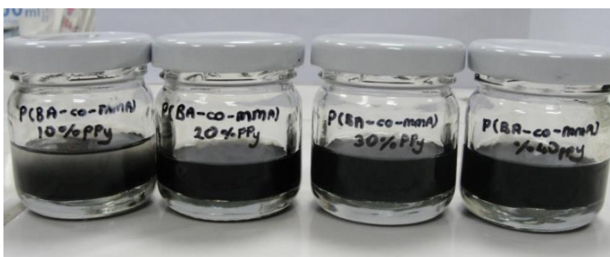
Figure 3.6: Composites with different polypyrrole composites
