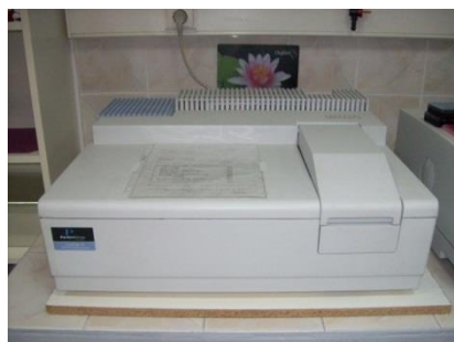
Figure 3.14: Perkin Elmer UV Visible Spectrophotometer.
