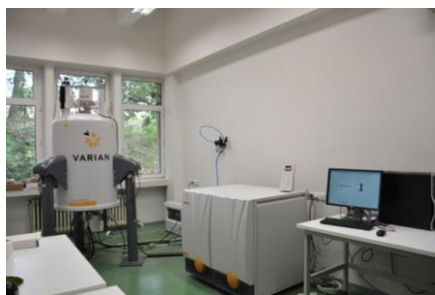
Figure 3.12: Agilent VNMRS 500 MHz Nuclear Magnetic Resonance Spectrometer
