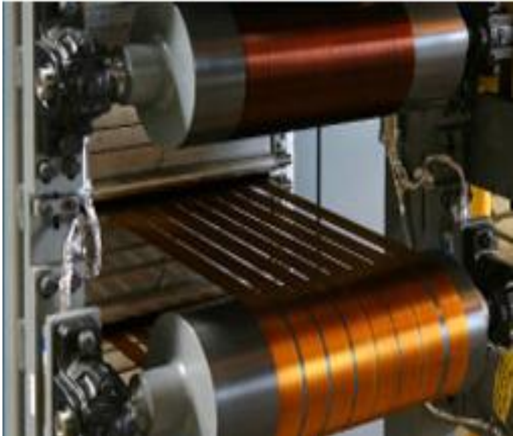
Figure 2.7 : Stabilization furnace and oxidized PAN fibers [18]
