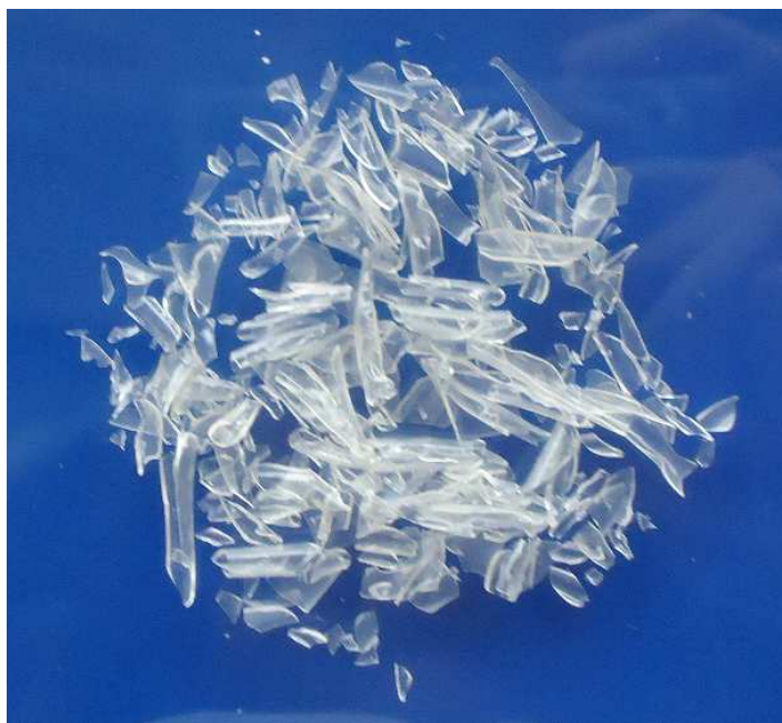
Figure 4.18 : Film CSPU-2 after the sunlight exposure
