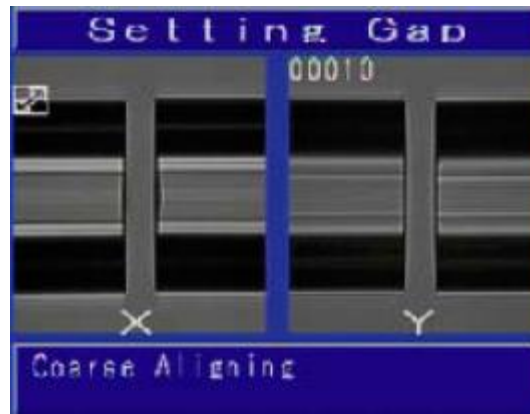
Figure 4.2: Alignment of fiber ends in three axes
