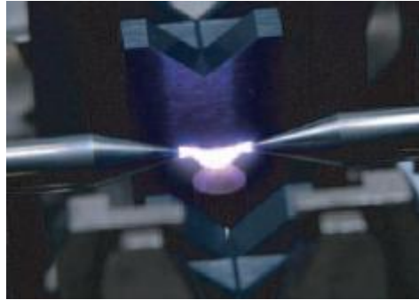
Figure 4.1: Arc generated by a fusion splicer
