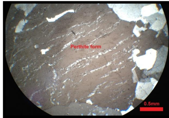
Figure 4.12 : Thin section photograph is showing Biotit-granite from Eybek granodiorite with Perthite texture from a metaluminous biotite granite. The lighter irregular stripes and patches of bright yellowish-white albite between dimmer gray stripes and patches of microcline. The color difference is mostly caused by the different optical orientations of the two different minerals in cross polarized light.(sample no:20 in table).
