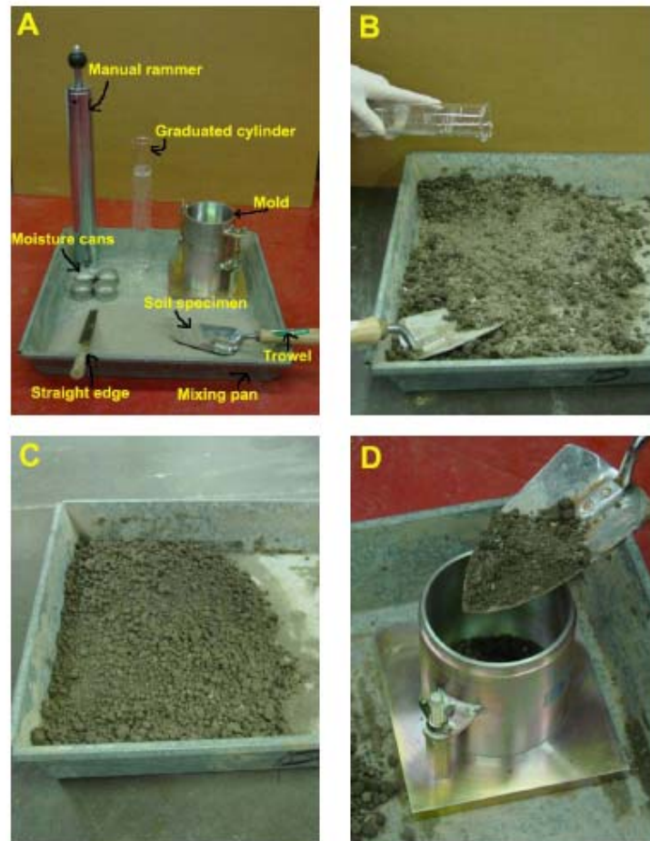
Figure 3.7 : Compaction Step – I [4].
