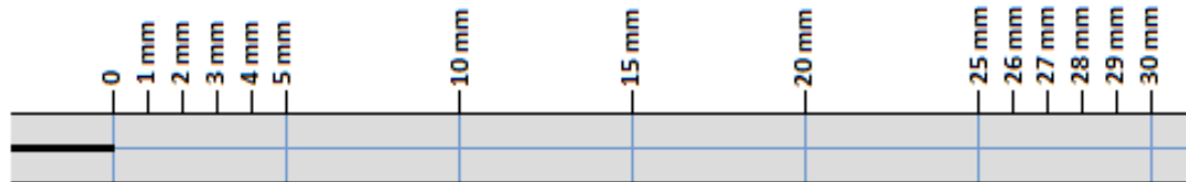
Figure 3.23 : Delamination propagation marking
