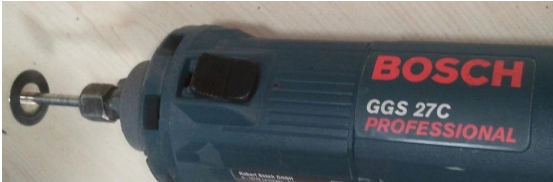
Figure 3.14 : Hand held power tool used for cutting plates
