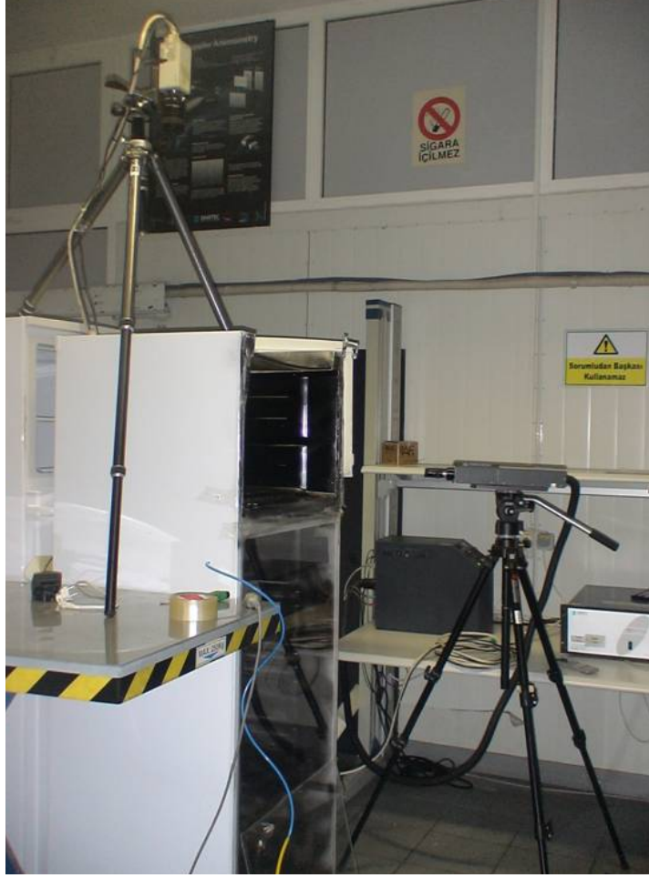
Figure 3.5: The experimental setup for PIV
