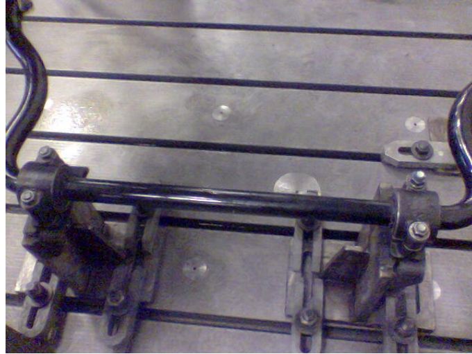
Figure 4.4: Stabilizer is also fixed around the both bearings along its axis.
