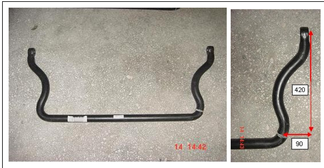
Figure 7.1: Stabilizer Bar – Vertical and horizontal distances of fracture point from the axis of movement (used in formula, See Table 7.1)
