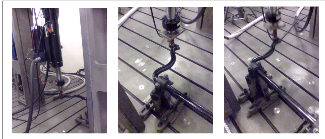
Figure 4.1: Stabilizer bar supported at one end and forced at the other one.
