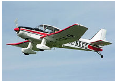
Figure 2.1: Conventional landing gear of a SAN Jodel D.140 Mousquetaire [9].
