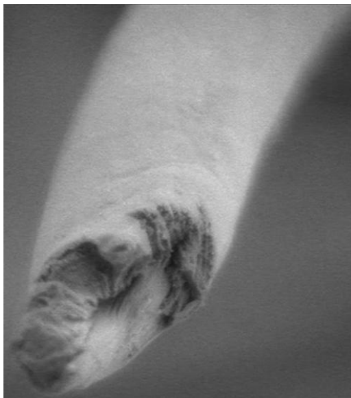
Figure 4.105 : Tensile break of sample 235.
