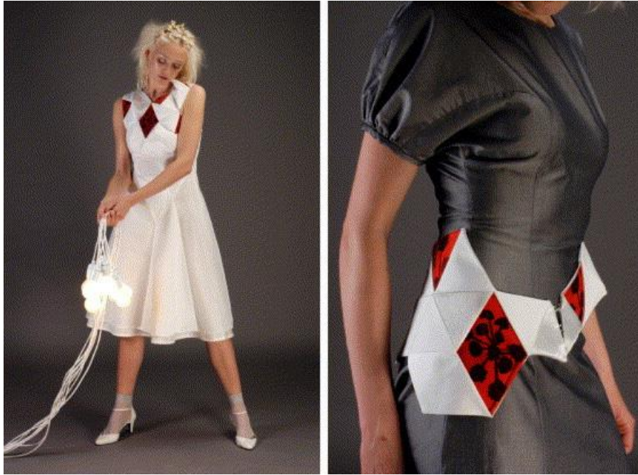
Figure 1.14 : Organic polymer solar cells integrated into clothes (Krebs, 2006).
