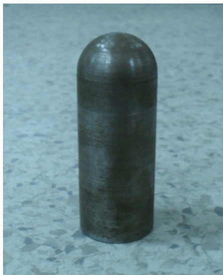
Figure 5.3 : Metal dome probe.
