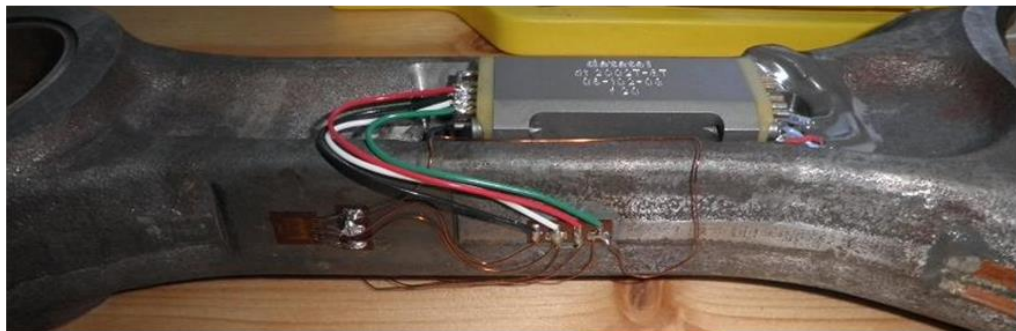
Figure 3.19 : Instrumentation of strain gages and connections to the transmitter.
