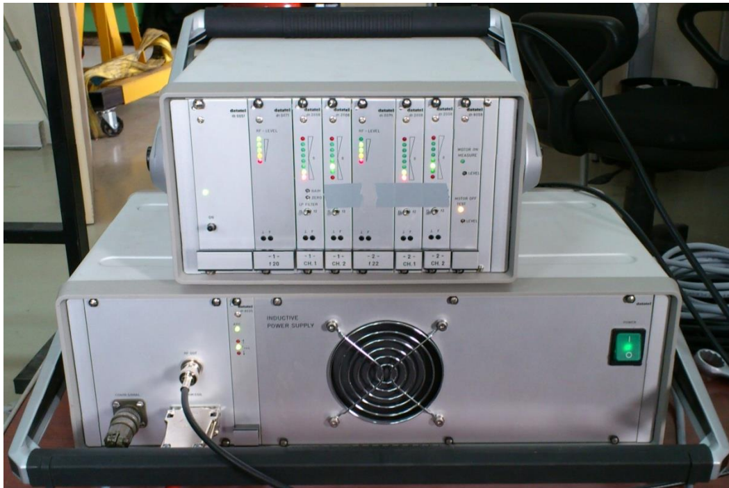
Figure 3.3 : Receiver and inductive power generator units.
