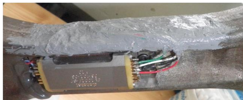
Figure 3.20 : Using adhesives to cover the cables.
