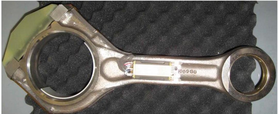
Figure 3.1 : Connecting rod with transmitter and rotor coil units.
