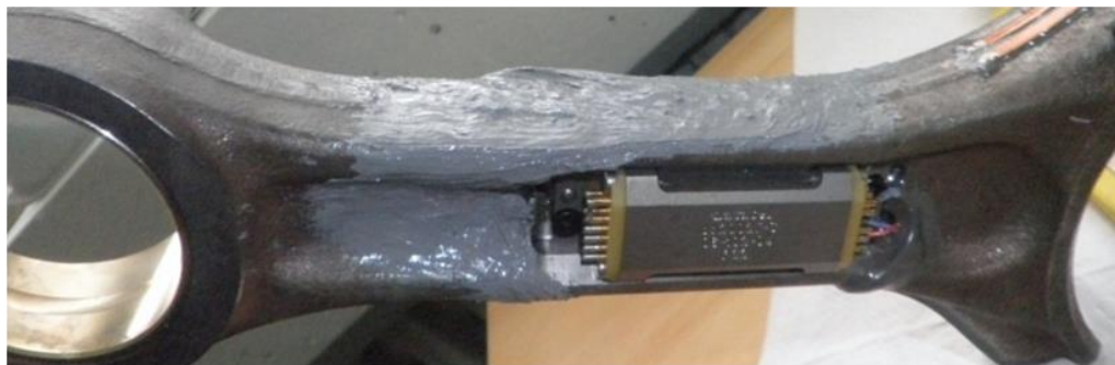
Figure 3.19 : Instrumentation of strain gages and connections to the transmitter.
