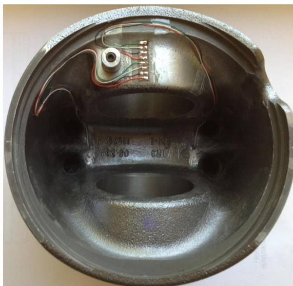
Figure 3.15 : Placement of sensor cables and terminal for cable connections.
