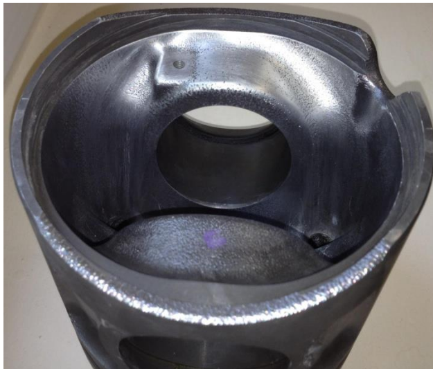
Figure 3.14 : Smoothing the surface inside the piston with sandpaper.
