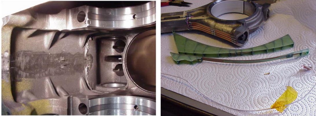
Figure 3.36 : Engine block surface after smoothing and antenna brackets.
