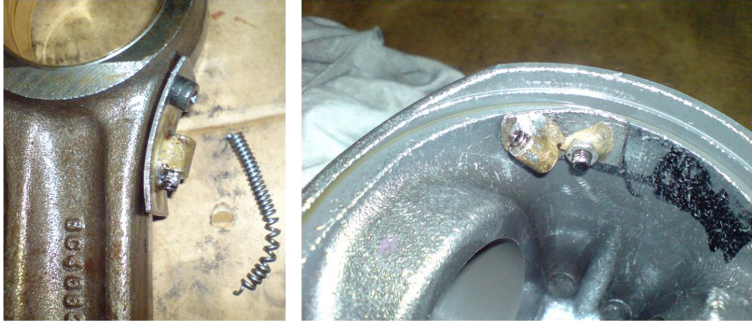
Figure 3.22 : The condition of Bowden cable design after testing.
