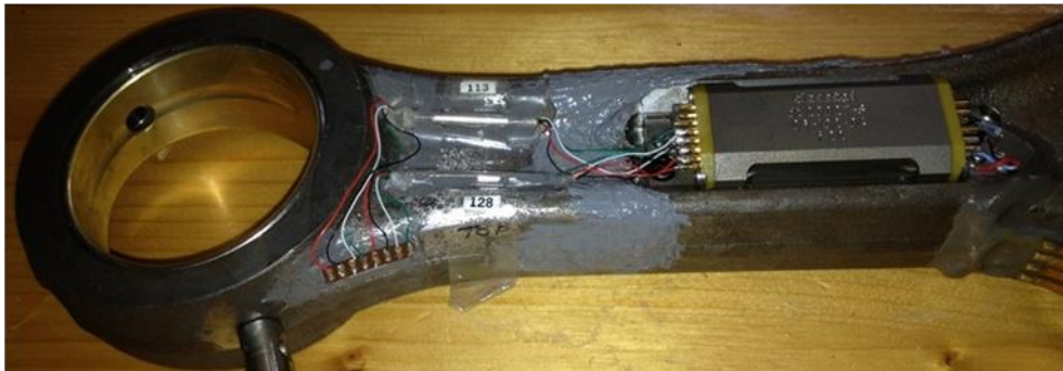
Figure 3.21 : Placement of pressure sensor bridges.
