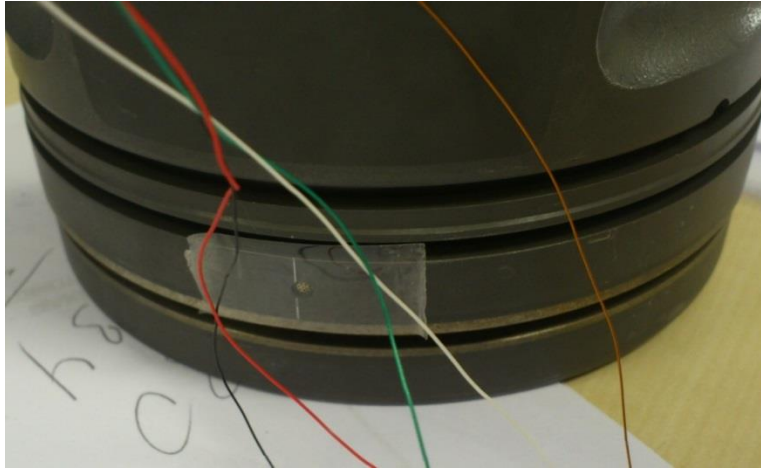
Figure 3.13 : Placement of sensors inside the piston.
