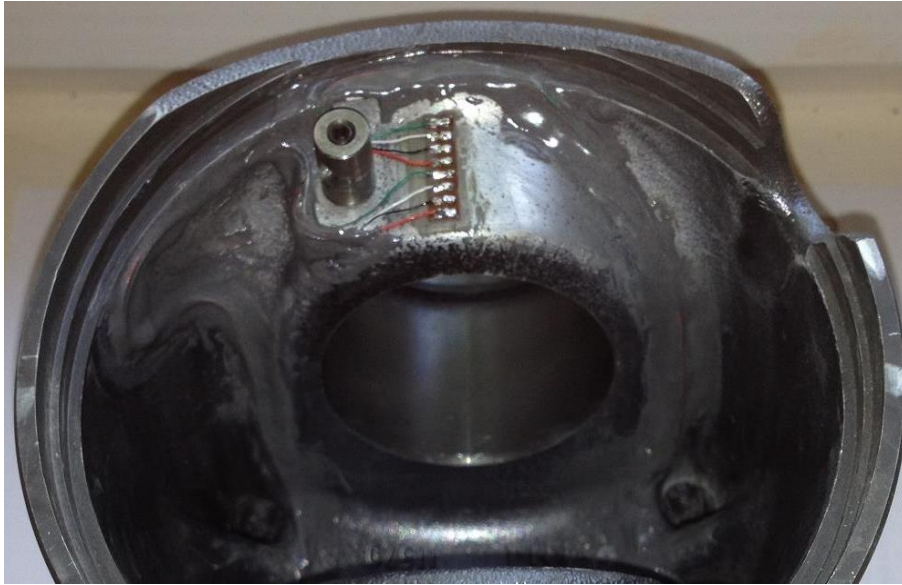
Figure 3.16 : Covering up the cables using JB Weld.
