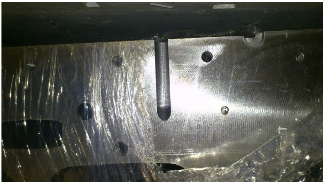
Figure 3.39 : Small machining at block underside to take out stator coil cables.
