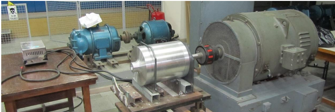
Figure 3.32 : Motor test bench.
