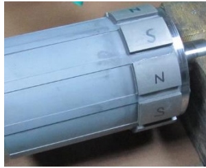
Figure 3.21 : Magnet attachment process.
