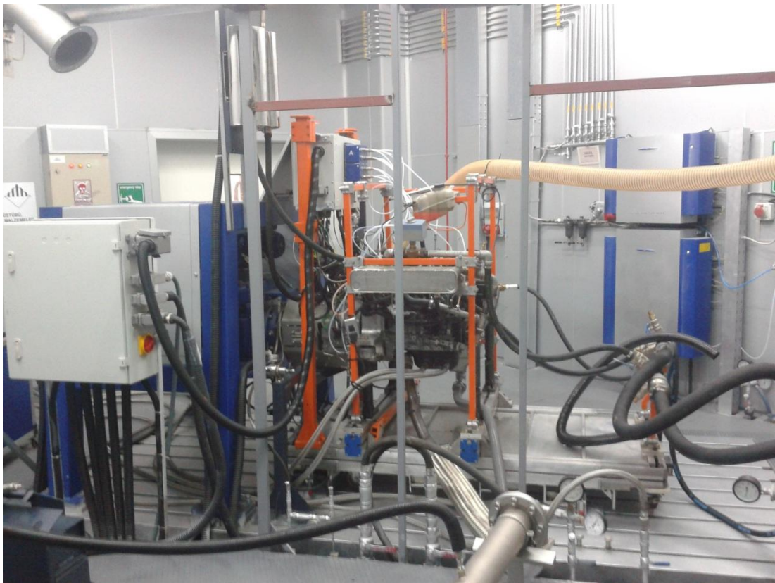
Figure 4.1 : The test cell used for the P&E calibration.
