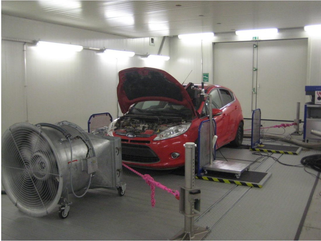
Figure 4.19 : Emission test at the chassis dynamometer.
