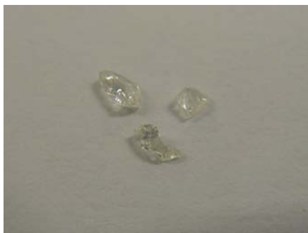
Figure 4.9 : As-cast 0.70 GeO 2 – 0.30 PbF 2 binary glass samples.
