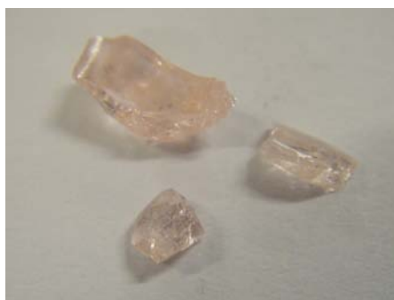
Figure 4.29 : As-cast 0.78 GeO 2 – 0.20 PbF 2 – 0.02 Er 2 O 3 glass samples.
