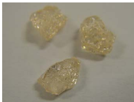
Figure 4.21 : As-cast 0.695 \text{ GeO}_2 - 0.30 \text{ PbF}_2 - 0.005 \text{ Er}_2\text{O}_3 glass samples.
