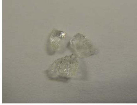
Figure 4.5 : As-cast 0.80 GeO 2 – 0.20 PbF 2 binary glass samples.
