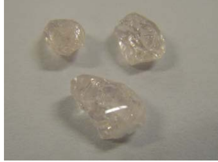
Figure 4.13 : As-cast 0.895 GeO 2 – 0.10 PbF 2 – 0.005 Er 2 O 3 glass samples.
