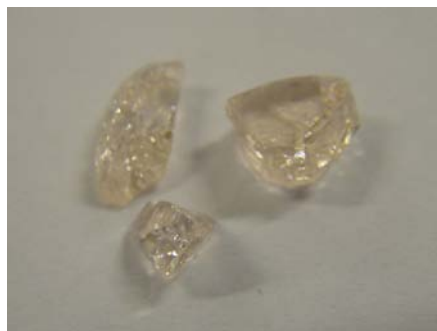
Figure 4.17 : As-cast 0.795 \text{ GeO}_2 - 0.20 \text{ PbF}_2 - 0.005 \text{ Er}_2\text{O}_3 glass samples.
