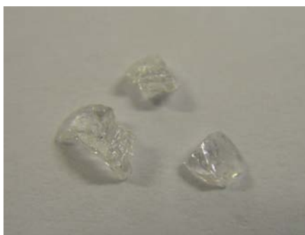
Figure 4.1 : As-cast 0.90 GeO 2 – 0.10 PbF 2 binary glass samples.
