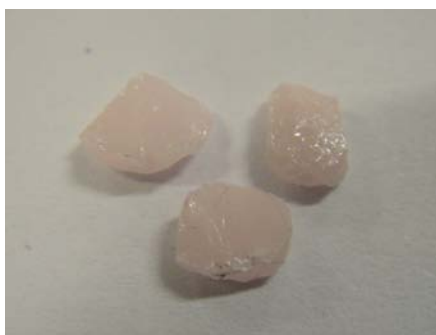
Figure 4.25 : As-cast 0.88 \text{GeO}_2 – 0.10 \text{PbF}_2 – 0.02 \text{Er}_2\text{O}_3 glass samples.
