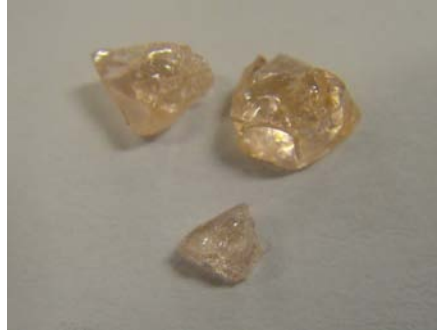
Figure 4.33 : As-cast 0.68 \text{ GeO}_2 - 0.30 \text{ PbF}_2 - 0.02 \text{ Er}_2\text{O}_3 glass samples.
