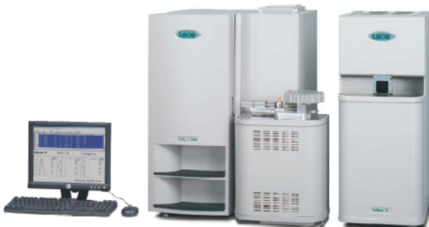
Figure 5.2 : A Leco TruSpec® CHN model instrument with a Leco TruSpec® S module for elemental analyses.
