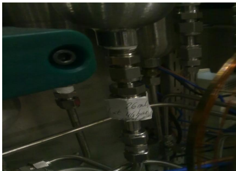
Figure 3.9 : Orifice for mass control of the Ar feed.
