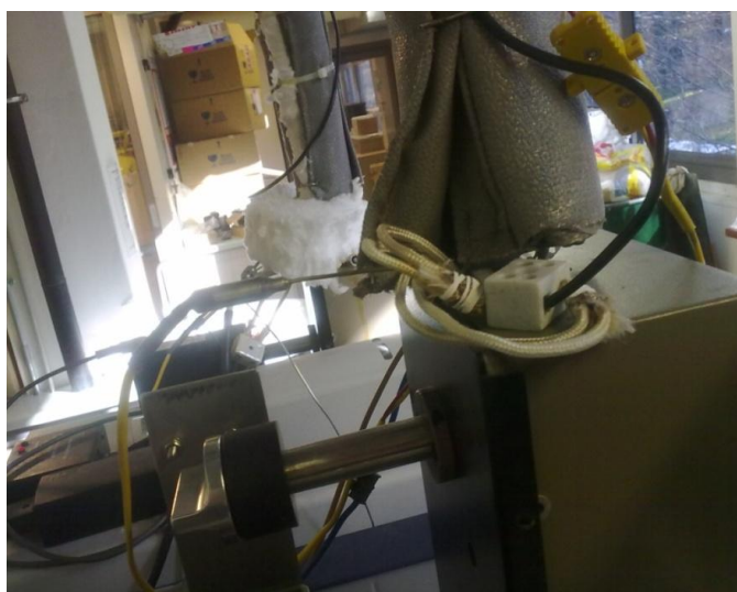
Figure 3.1 : Rotating valve for GC analysis.
