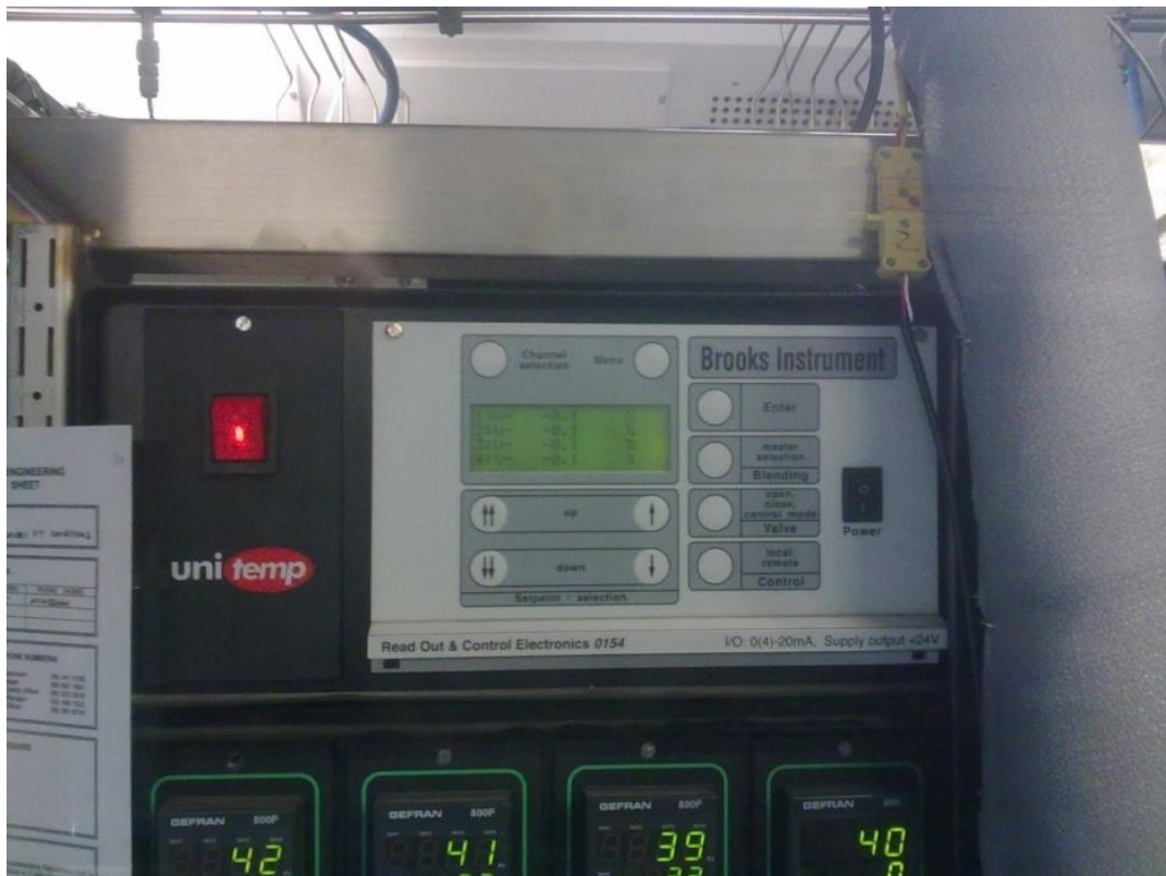
Figure 3.6 : Electronic interface of the master controllers.
