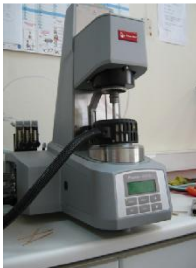
Figure 7.1 : A photo of rotational rheometre MCR 301
