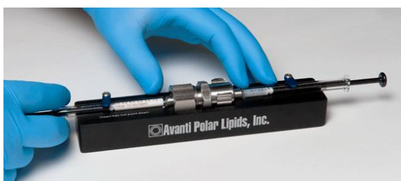
Figure 3.3 : Representation of using of Avanti Mini Extruder to make homogenized vesicles.
