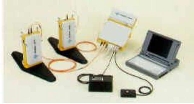
Figure 2.5. Components of a GPR system. Unshielded, bistatic, dipole antenna with its control unit and recording notebook computer.
