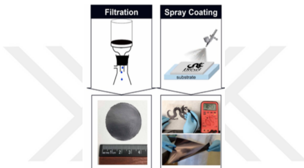
Figure 2.16. Coating methods of mxene powders onto substrates. [33]
