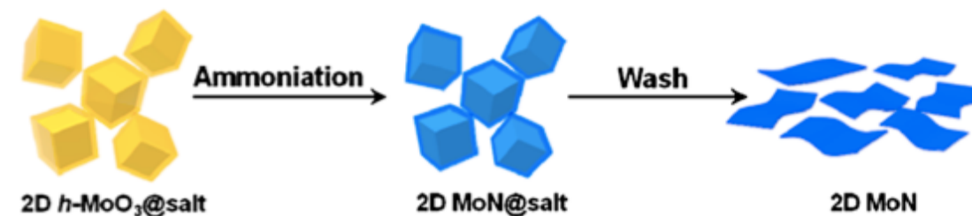
Figure 2.13. Mxene production by template method. [31]
