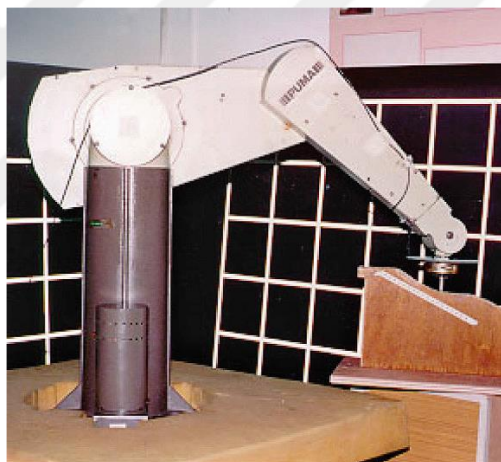
Figure 1.4 : PUMA (Programmable Universal Machine for Assembly) robot [10].
