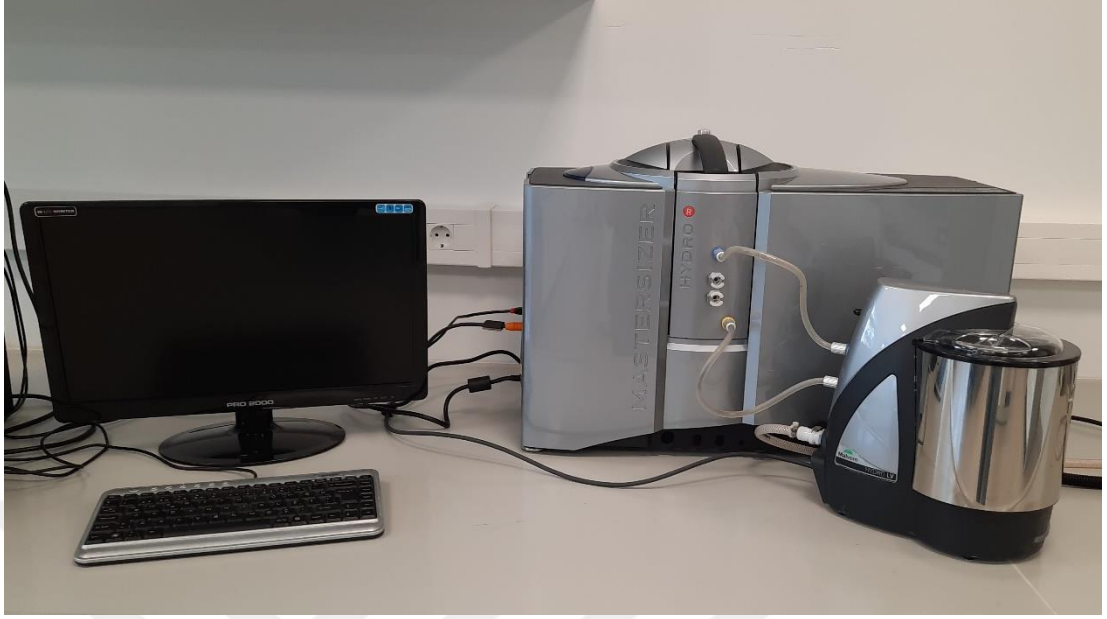
Figure 3.4 : MALVERN Mastersizer Laser Particle Size Analyzer provides particle size measurements.
