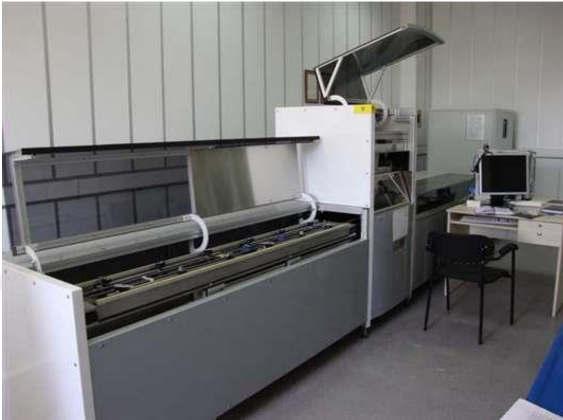
Figure 3.6 : ITRAX XRF Core Scanner provides elemental analyses on sediments core with high resolution. Instrument also provides optical and radiographic images. Study contains elemental distributions, which is provided in 1 mm measurement interval.
