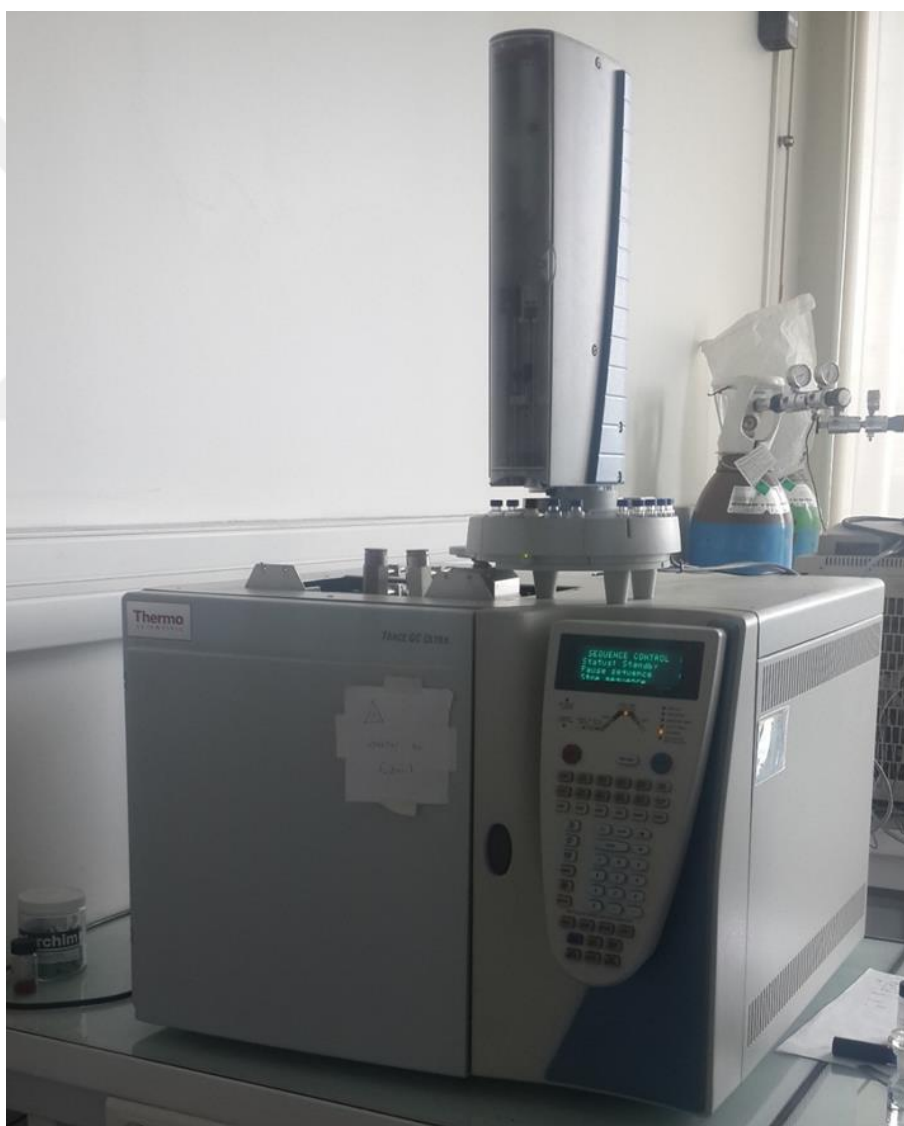
Figure 3.7 : Thermo Fisher Trace Ultra Gas Chromatograph (GC) analyzer provides the C37 unsaturation index ( UK'37 = C37:2 / (C37:2 + C37:3) ), leading to sea surface temperature (SST) record.
