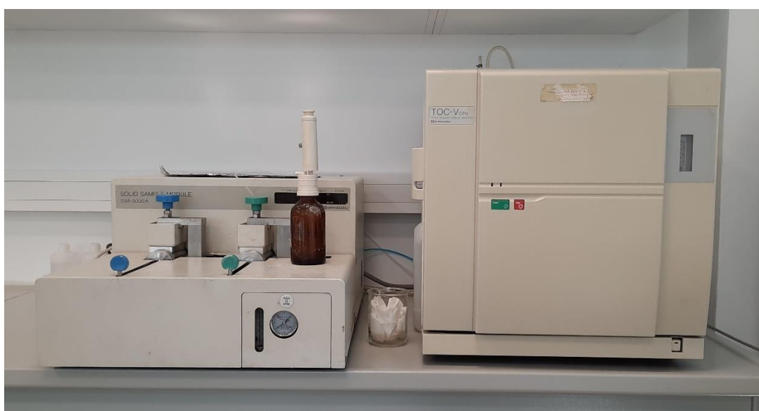
Figure 3.5 : Shimadzu TOC/TIC analyzer provides the information about the TOC content of sediments.
