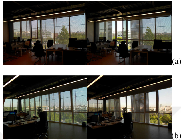
Figure 3.10 : The offices in ITU Lecture Hall A Building: (a) The intermediate office B22 on 2 nd floor with exterior movable metal panels as closed (left) and open (right), (b) The corner office B411 on 4 th floor with exterior movable panels as closed (left) and open (right).
